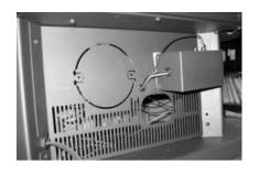
Remove the Heat Shield from the DC Spark Box.
